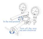
Record Obar record and close the relieve valve. Providing pressure about 4 bar by hand pump up and down,then adjust the F-adjust valve to second standard point(5bar).
