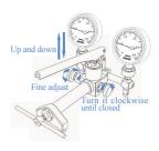
Rotate the lead screw clockwise to make pressure value close to next standard points, and adjust F-adjust valve to get exact values. Pressure rising&stabilize to 10bar,15bar,20bar,25bar in turn. Meanwhile, record the data.
