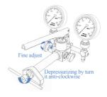
Finish the Loop calibration and open the relieve valve to release the pressure.
